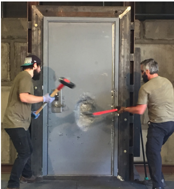
Image from actual forced entry testing
